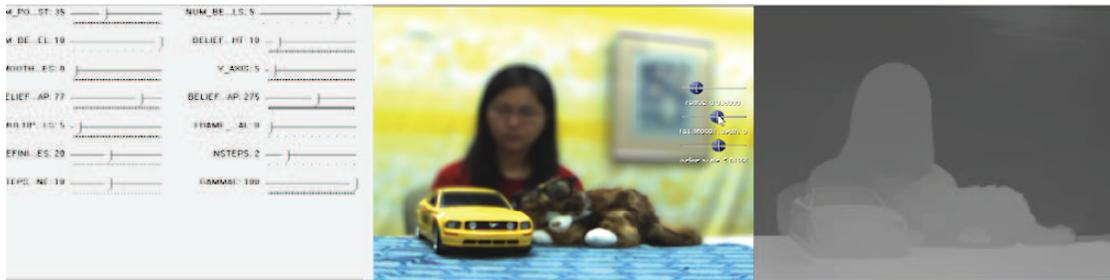
**Fig. 13** The real time DoF effects (middle) and disparity map (right) given by our system after fine tuning the parameters using our interface (left).
