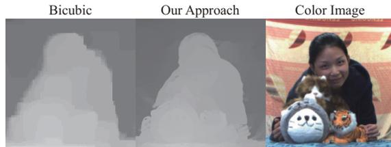
**Fig. 7** Comparison between our method and bicubic upsampling on real scenes. The disparity map is upsampled from  $320 \times 240$  to  $640 \times 480$ . Our method preserves sharp edges and maintains smoothness, which is critical to reliable DoF synthesis.
