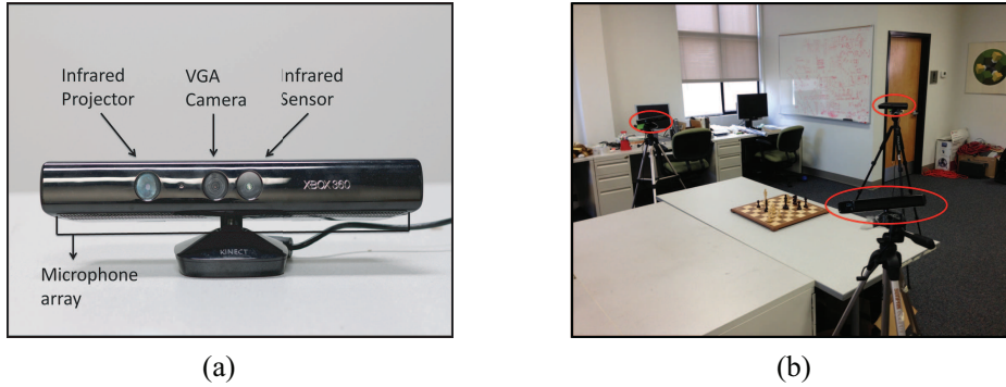
Figure 2. (a) Microsoft Kinect has a microphone array, an infrared projector, an infrared sensor and a VGA camera. (b) Acquisition system consists of a set of three Microsoft Kinect cameras.
