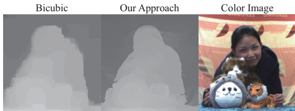
Fig. 5 Comparison between our method and bicubic upsampling on real scenes. The disparity map is upsampled from 320 \times 240 to 640 \times 480 . Our method preserves sharp edges and maintains smoothness, which is critical to reliable DoF synthesis.
