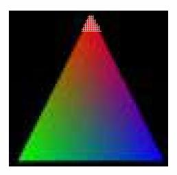
Triangle ~3,042 pixels Each pixel processed by fragment processor each frame
