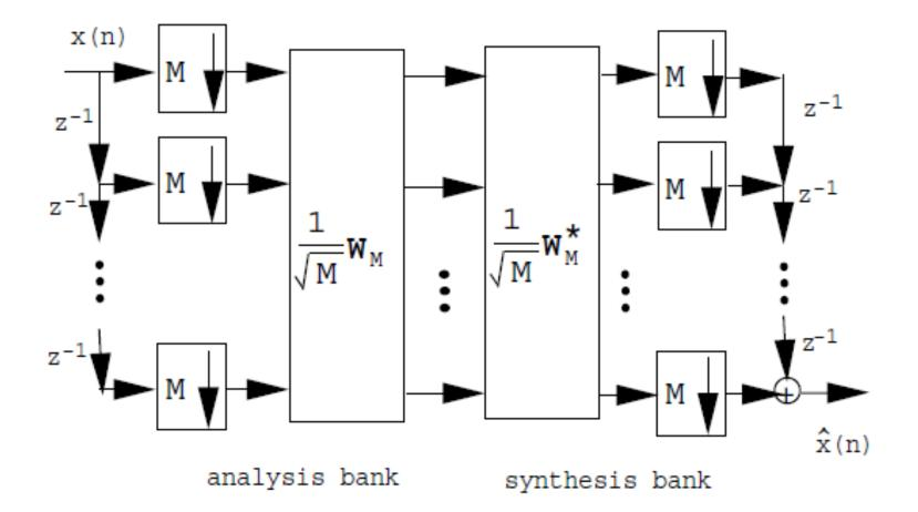
Figure 22: DFT (analysis bank) and IDFT (synthesis bank).
