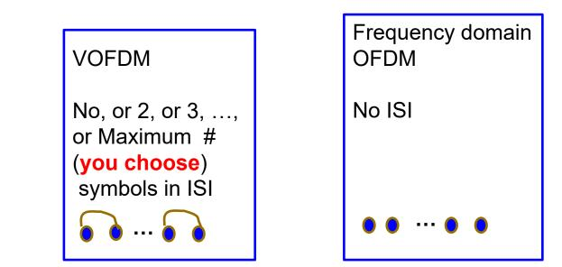
Single antenna VOFDM is in the middle between single carrier and OFDM in terms of dealing with ISI
