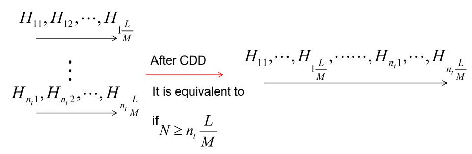
The number of multipaths is equivalently reduced by *M* times for VOFDM with a vector size *M*
