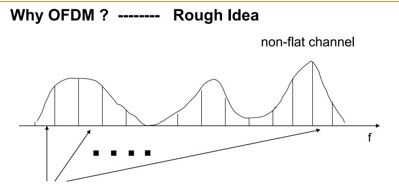
Narrow subchannels using multiple subcarriers
