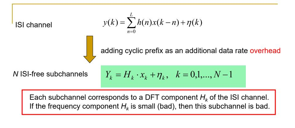
For 20 MHz Channel, $L \le 16$ OFDMN=64 $\Gamma=L=16$ , 25% data rate overhead
