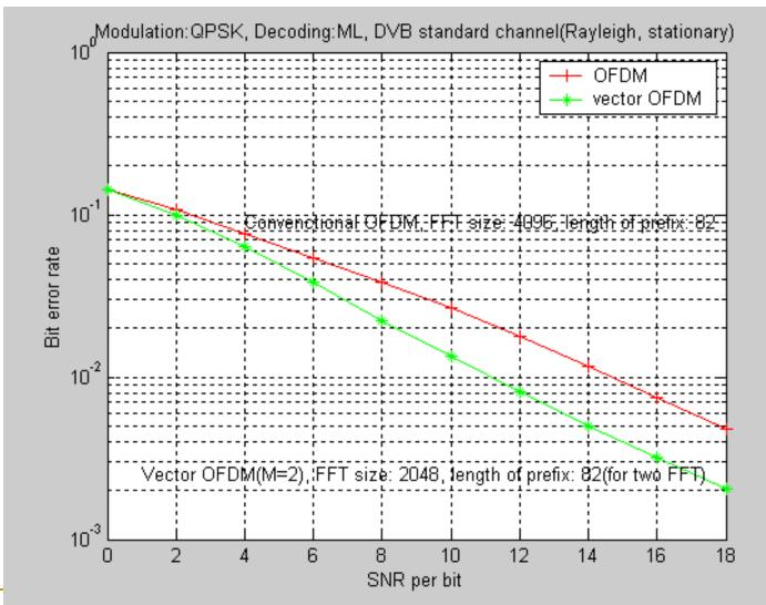
CP data rate overhead is the same for the two curves, matrix modulation is not used.
