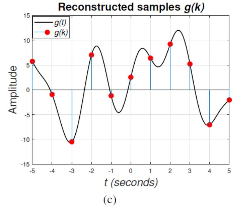
An example of digitizing  $x(t)$  with a 2-channel SR-ADC system. Here,  $m= 0.8$ ,  $\Delta_0 = 0.8 \cdot 5 = 4$  and  $\Delta_1 = 0.8 \cdot 6 = 4.8$ . The Nyquist sampling period is  $1 s$ . (a) and (b) show the outputs of the 1st and the 2nd channels, respectively. (c) shows the reconstructed values
