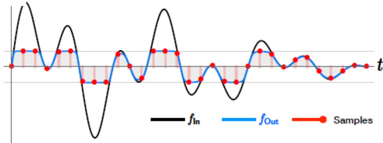
(d) Input Signal, Output Signal and Modulo Samples with Self-Reset ADC
