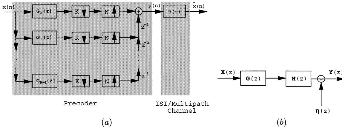
Fig. 1. (a) Filterbank precoding. (b) A general filterbank precoded system of matrix form.
