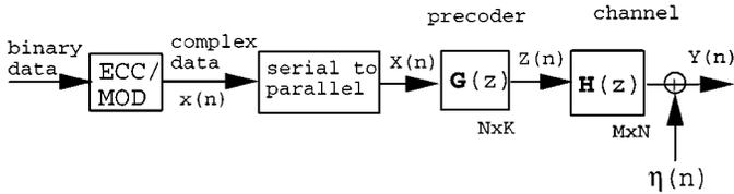
Fig. 5. An equivalent undersampled antenna array system.
