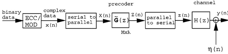
Fig. 2. A single-receiver communication system with baud-rate sampling.
