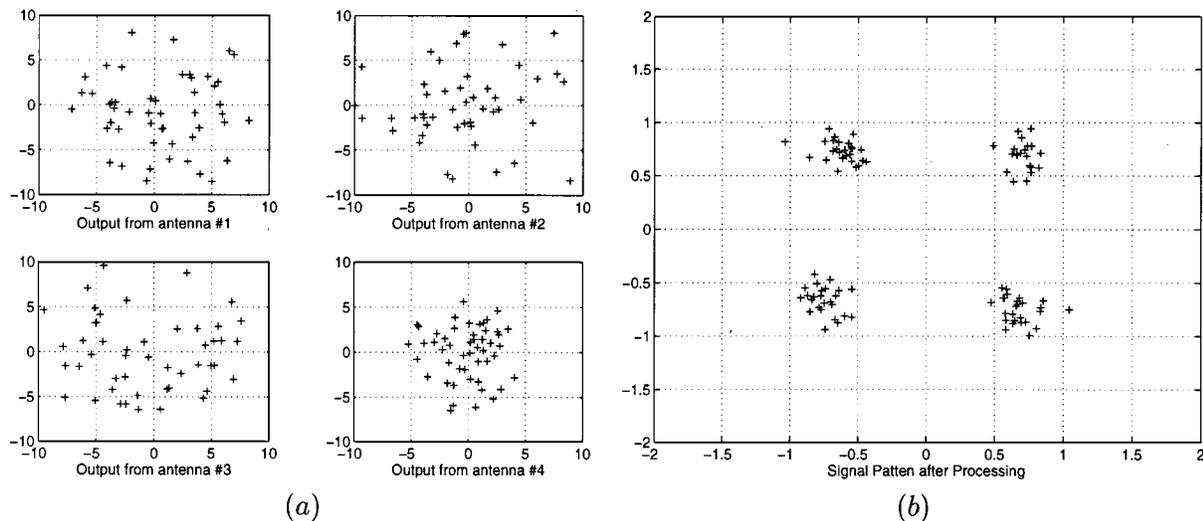
Fig. 8. (a) Undersampled antenna outputs before blind identification. (b) Recovered signal after blind identification using precoding techniques.
