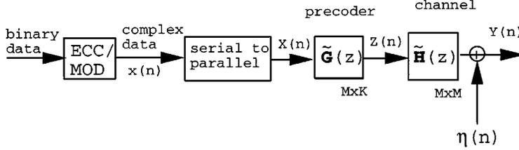
Fig. 3. A blocked single-receiver system with baud-rate sampling.
