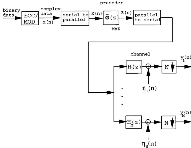
Fig. 4. An undersampled antenna array system.
