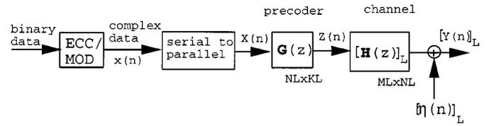
Fig. 6. A blocked undersampled antenna array system.
