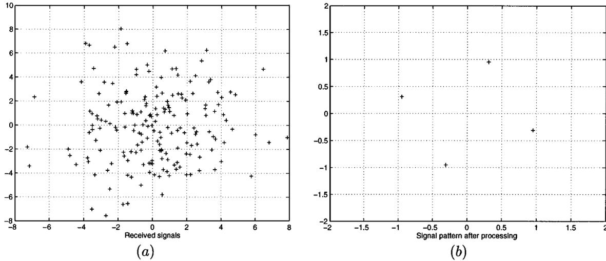
Fig. 7. (a) ISI channel outputs with baud sampling; (b) recovered signal after blind identification using precoding techniques.
