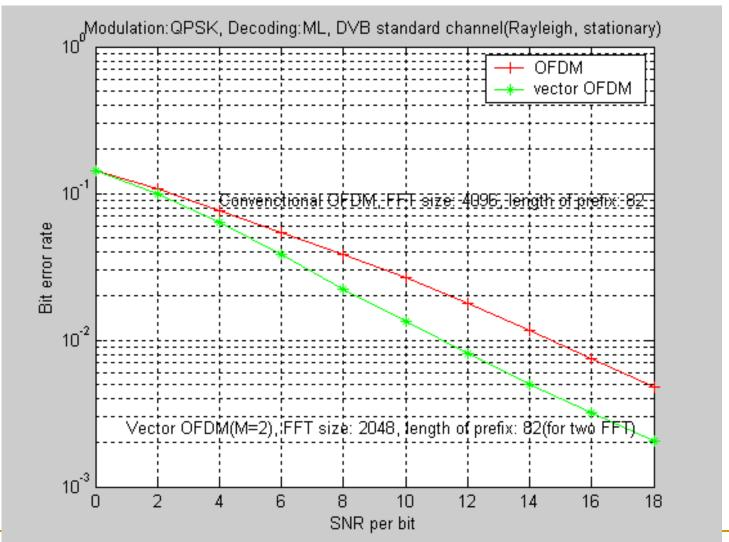
CP data rate overhead is the same for the two curves, matrix modulation is not used.
