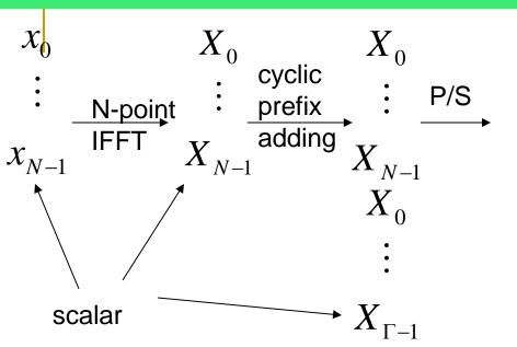
OFDM, when data rate overhead  $\Gamma \geq L$
