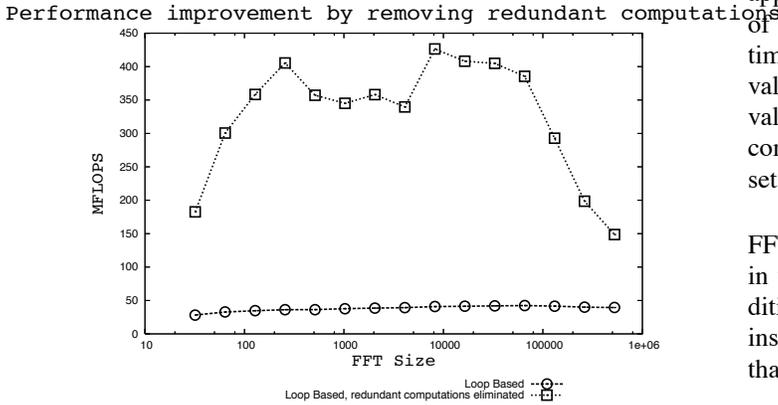
Figure 3: Improvement after removal of redundant computations
