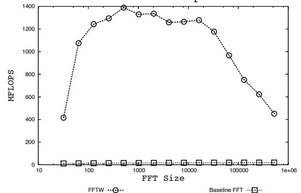
**Figure 1:** Comparison between a simple implementation of FFT and the commercial FFTW
