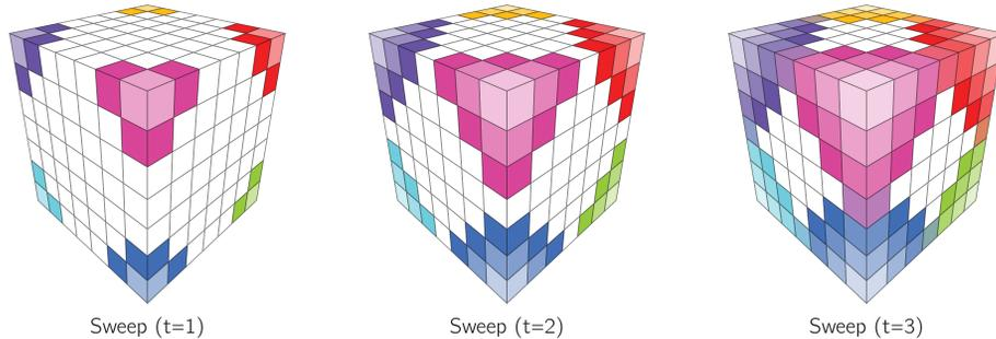
Time sequence of the sweep kernel ( $H^{-1}$ ) moving through the mesh. Multiple sweeps can occur at the same time. Grid contention occurs when a location has equal manhattan distance from two or more sources (corners).
