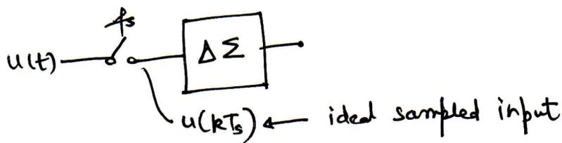
jittery sampled input =  $u(kT_s + \Delta t_k) \approx u(kT_s) + \Delta t_k \cdot \left. \frac{du}{dt} \right|_{t=kT_s}$
