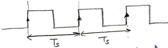
• Real oscillator →  $T_s$  is not constant from cycle to cycle
