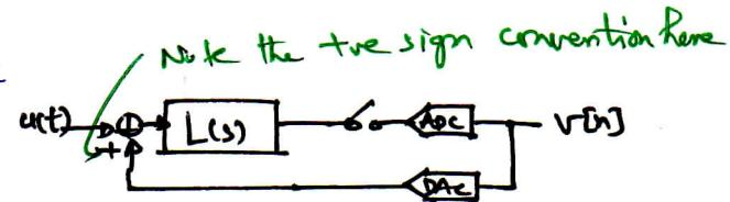
$$\Rightarrow L(s) = -\frac{1+1.5s}{s^2}, \quad L(z) = \frac{-2z+1}{(z-1)^2} \text{ with } \hat{\delta}_s(t) = (\alpha, 1) \quad \text{E DAC pulse shape}$$
