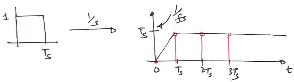
$\Rightarrow$  for sampling rate  $f_s > 1$ , the pulse shape width is reduced
