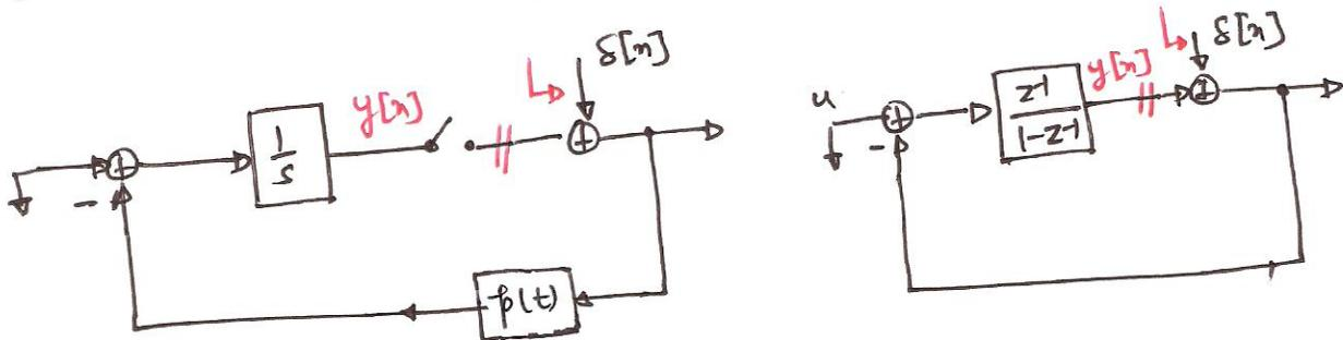
• If a DT impulse is launched after the sampler, then the returned response after the sampler should be equal to the impulse response in DT modulator.
