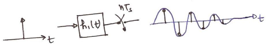
Can use a continuous-time (CT) impulse response  $h_c(t)$  such that the sampled response is  $h[n]$ .
