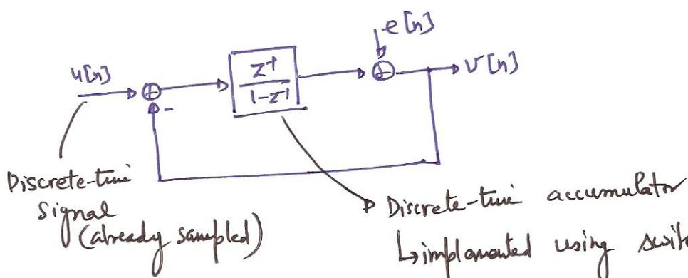
↳ implemented using switched capacitor circuits
