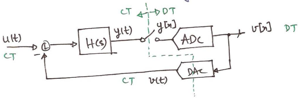
The loop filter is realized using CT circuitry, but made to look like a discrete-time loop-filter.
