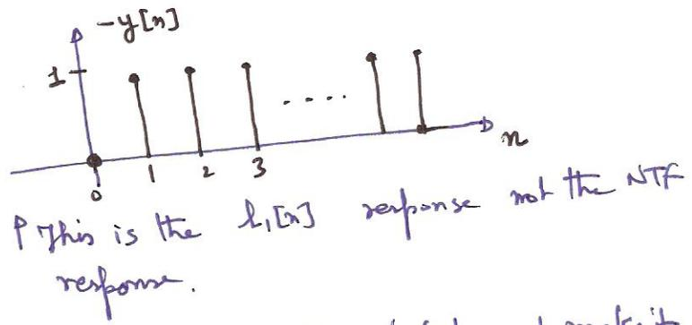
⇒ Rather than working with  $NTF(z) = \frac{1}{1-L_1(z)}$ , deal with  $L_1(z)$  and make it equal for DT as well as the CT ~~loop~~ loop.
