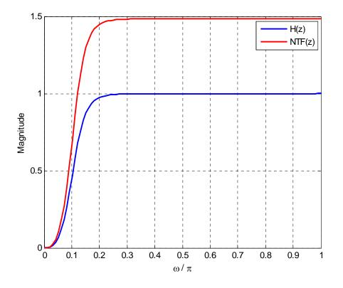
Start with cutoff frequency ω<sub>3dB</sub>=π/8, for the butterworth HPF H(z).
