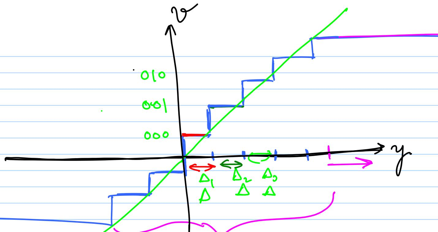
Uniform quantizer : fixed-level spacing ( $\Delta$ )
