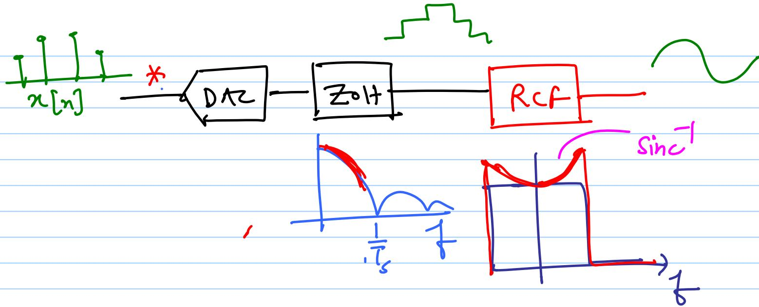
$\text{sinc}^{-1}$  response shape is used in the RCF to compensate for the sinc distortion in the ZOH.
