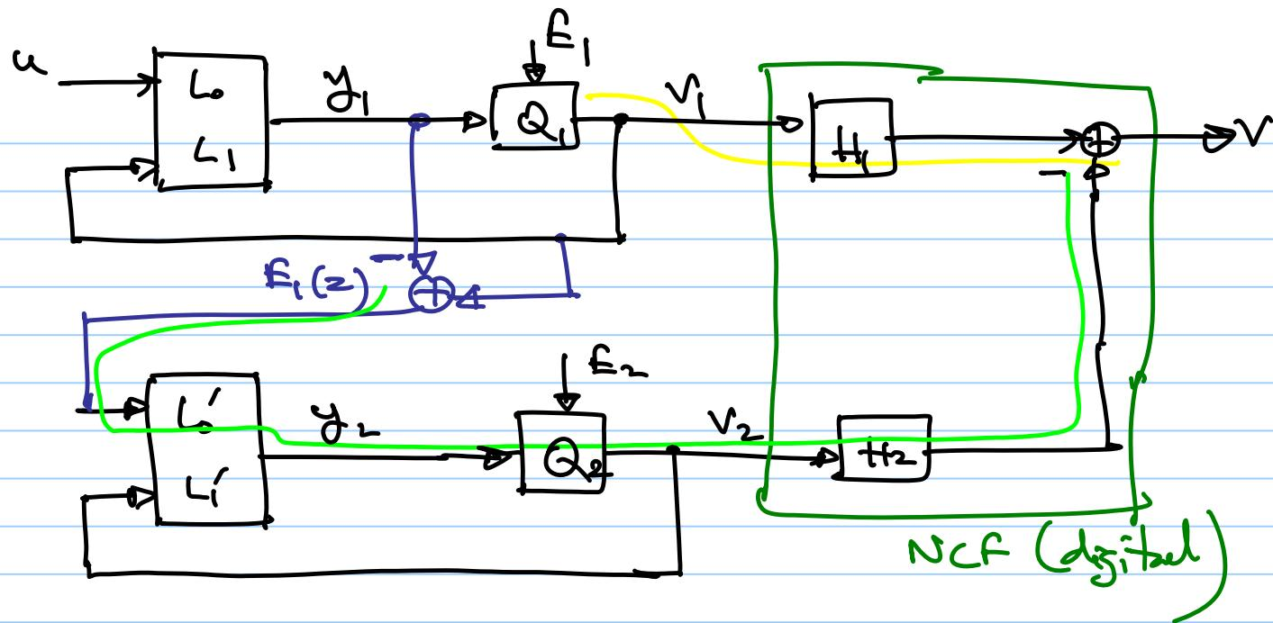
$$V(z) = H_1 V_1 - H_2 V_2$$
