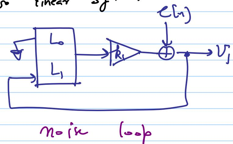
$$NTP'(z) = \frac{L_1(z)}{1 - k_1 L_1(z)} = \frac{NTF(z)}{k_1 + (1-k_1)NTF(z)}$$
