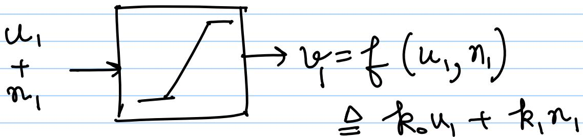
Approx. the quantizer by a two input linear system
