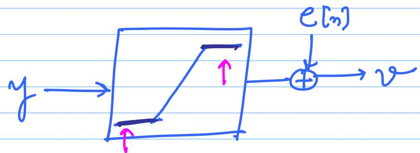
\* Overload (saturation) of the quantizer causes instability
