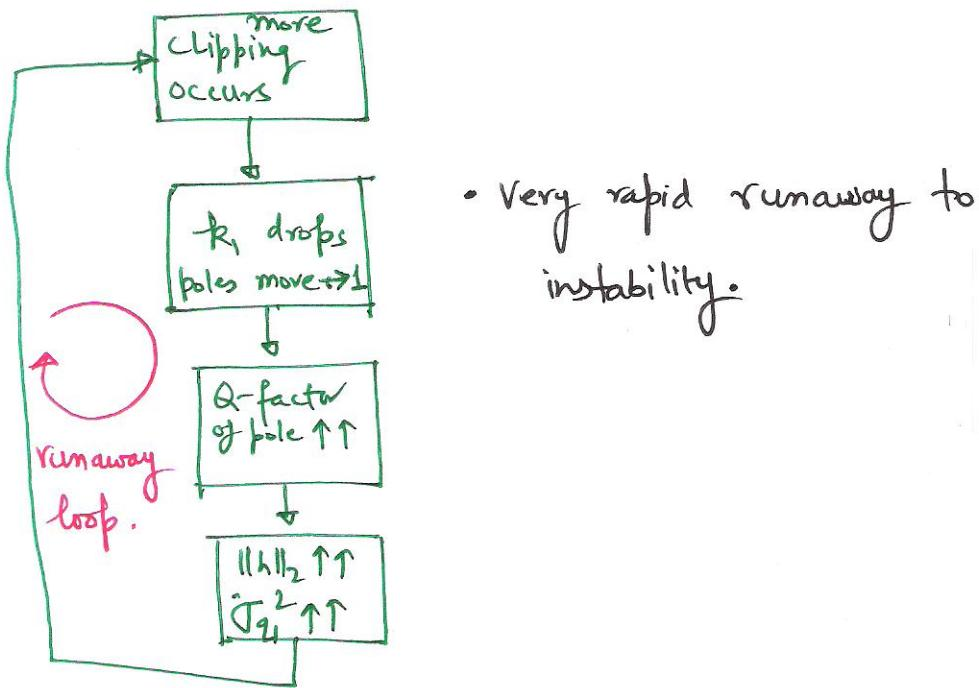
$\Rightarrow$  Modulator can not be stable for the signal level upto the saturation level of the quantizer. ( $MSA \Rightarrow$  maximum stable amplitude)
