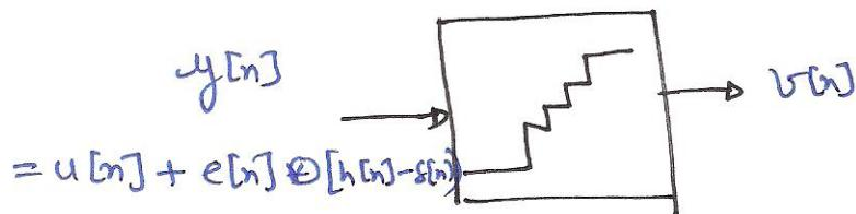
the sum of input and ~~step~~ quantization noise, shaped by the filter ( $h[n] - s[n]$ ) is quantized by the quantizer.
