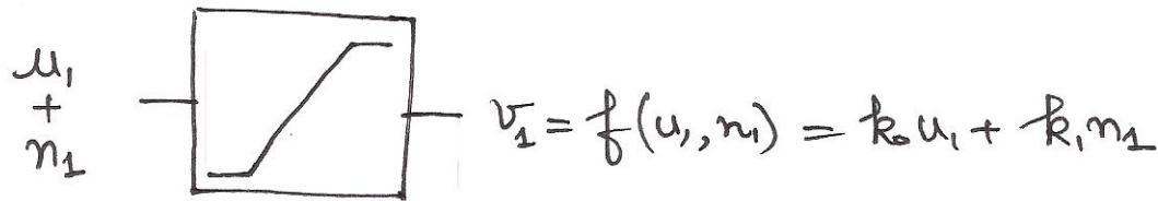
Approximating the quantizer by a two input linear system.
