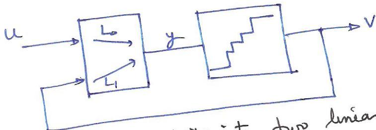
The modulator splits into two linear systems.
