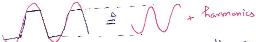
\* the gain for the input ( $u$ ) is the amplitude of the first harmonic of the clipped output. ( $k_0 \approx 0.9$ ) for  $A=1.2 \cdot f_s$
