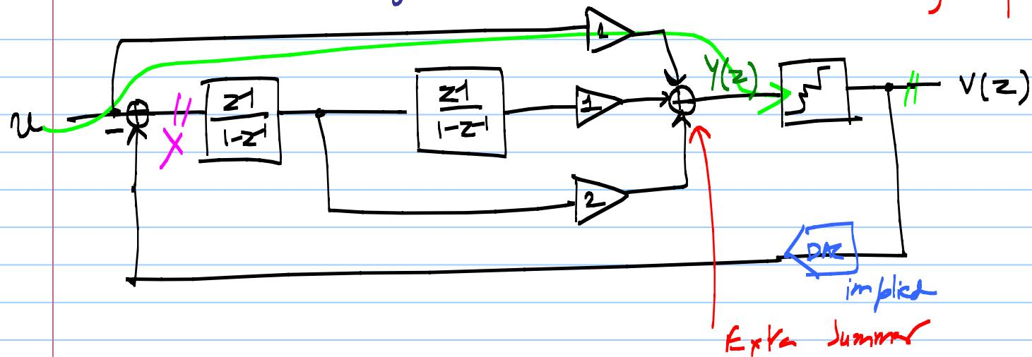
$$v(z) = \underbrace{u(z)}_{\text{STF}} + \underbrace{(1-z)^2}_{\text{NTF}} e(z)$$
