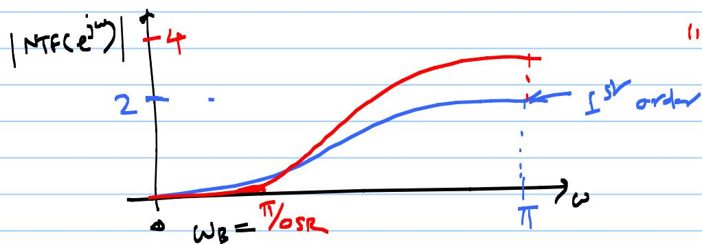
$$IB_N = \frac{\Delta^2}{2\pi} \int_0^{\pi/\text{OSR}} |(1 - e^{j\omega})^2|^2 d\omega$$
