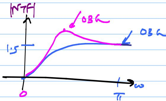
$$\begin{aligned} OBG &= \max_{\omega} |NTF(e^{j\omega})| \\ &= \text{infinity norm} \Rightarrow \|NTF\|_{\infty} \end{aligned}$$
