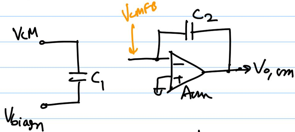
\*  $C_1$  is charged to  $V_{CM} - V_{biasn}$
