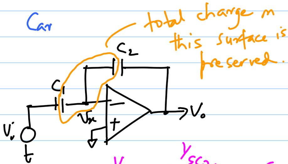
$$\frac{v_o}{v_i} = -\frac{v_{sc2}}{v_{sc1}} = -\frac{C_1}{C_2}, \quad \text{No resistive loading!}$$
