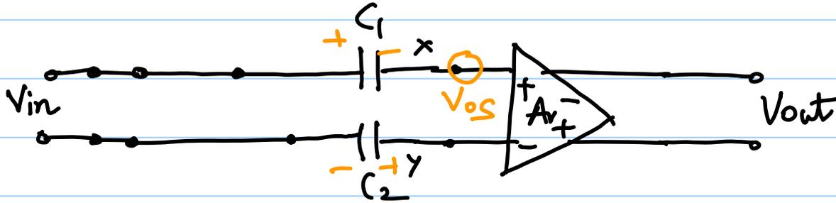
$$\begin{aligned} \frac{A_v}{1+A_v} V_{OS} - V_{OS} &= V_{OS} \left[ \frac{\cancel{A_v} - 1 - \cancel{A_v}}{1+A_v} \right] \\ &= -\frac{V_{OS}}{1+A_v} \approx -\frac{V_{OS}}{A} \end{aligned}$$
