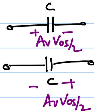
when all the voltages are settled,  $AvV_{os}$  is stored on the capacitors
