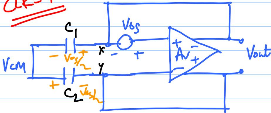
$$V_{out} = V_{xy}$$
