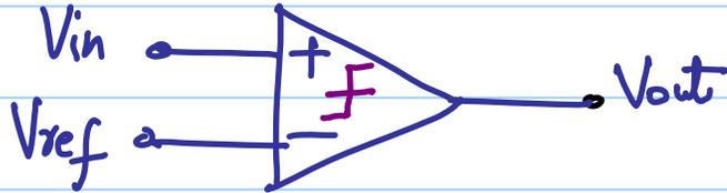
if  $V_{in} > V_{ref} \Rightarrow V_{out} = V_{DD}$
