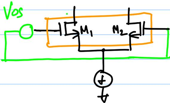
$$V_{os} = \Delta V_{THN} + \frac{1}{2} V_{ov} \cdot \frac{\Delta(W/L)}{W/L}$$
