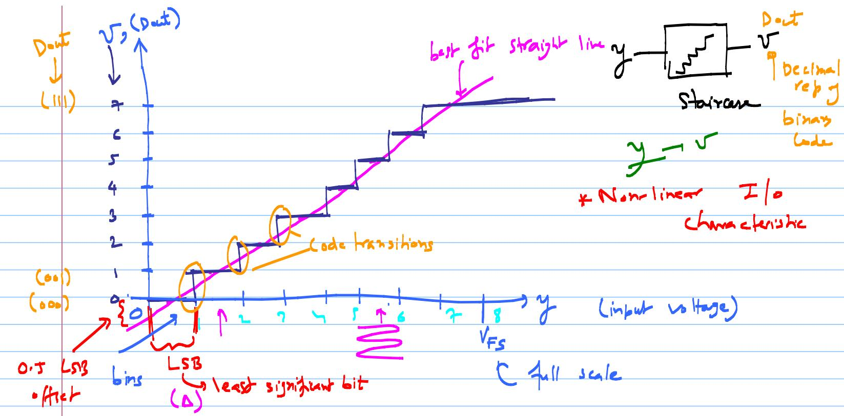
\* in an ideal quantizer, the code widths of all the bins
