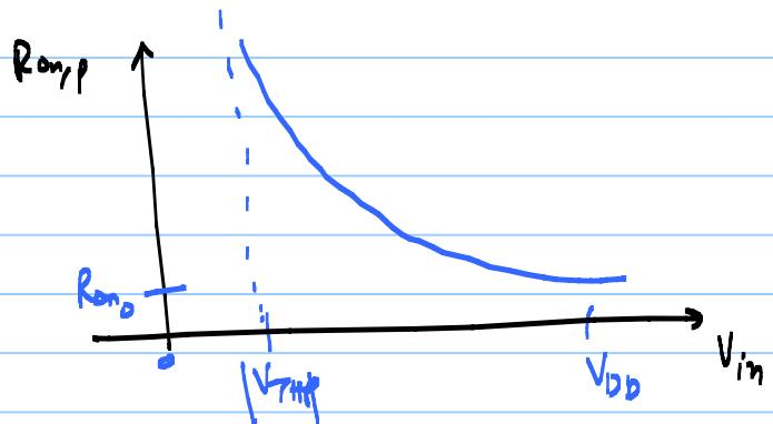
$$R_{on,P} = \frac{1}{\mu_p C_p \frac{W}{L} (V_{in} - |V_{THP}|)}$$
