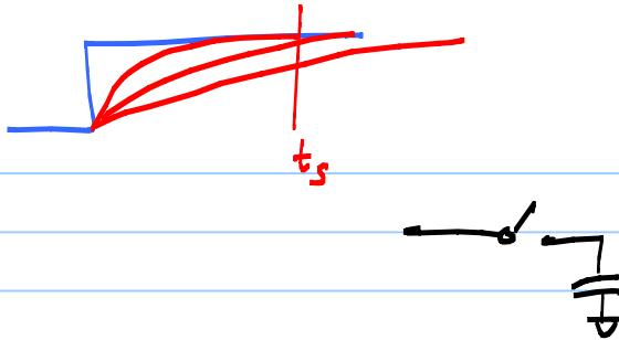
$$\frac{V_{out}}{V_{in_0}} = \left(1 - e^{-\frac{t}{\tau}}\right)^2$$
