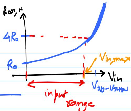
$$\frac{1}{R_{on,n}(V_{in,max})} = \frac{4}{R_0 + R_{on,n}(0)}$$
