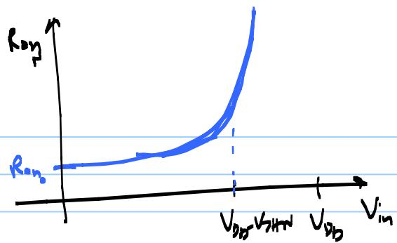
$$R_{on,N} = \frac{1}{\mu_n C_n \frac{W}{L} (V_{DD} - V_{in} - V_{THN})}$$
