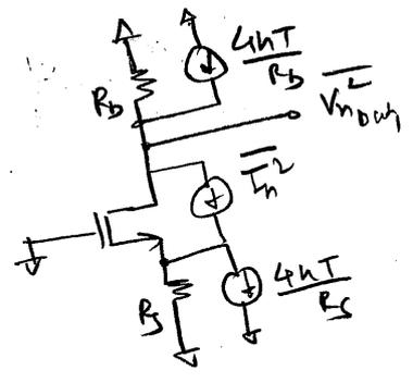
$$\overline{V_{n,out}^2} = 2 \times 4kT \times \left[ \frac{1}{R_B} + \frac{2}{3g_{m1}} \left( \frac{g_m}{1 + g_{m1}R_S} \right)^2 + \frac{1}{R_S} \left( \frac{R_S}{g_{m1} + R_S} \right)^2 \right] R_D^2$$
