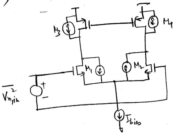
Noise current due to  $I_{bias}$  is CM at the output  $\Rightarrow$  no effect on  $V_{n,in}^2$
