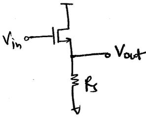
$$A_v = \frac{R_s}{\frac{1}{g_m} + R_s} = g_m \cdot (\frac{1}{g_m} \parallel R_s)$$
