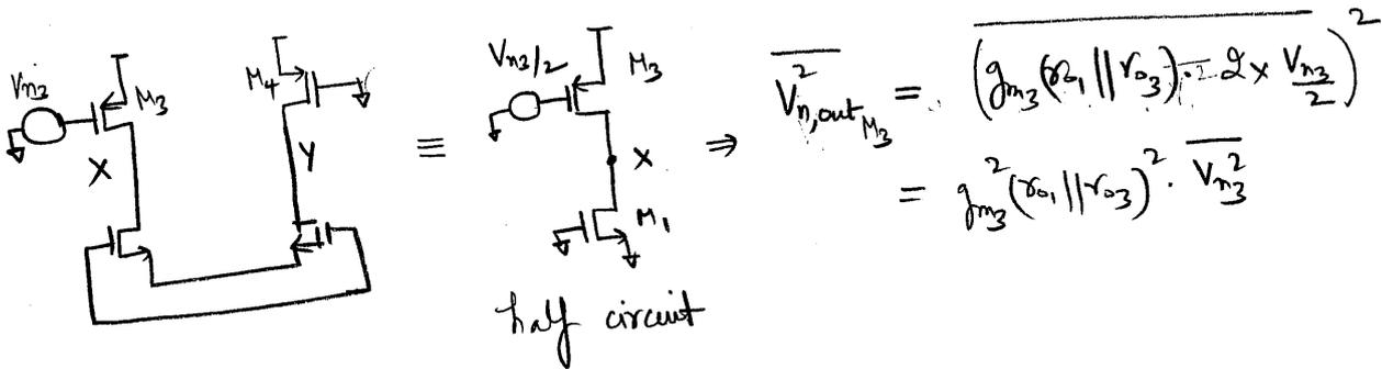
$$\begin{aligned} \Rightarrow \overline{V_{n,out}^2} |_{M_3, M_4} &= g_{m3}^2 (r_{o1} \parallel r_{o3})^2 \overline{V_{n2}^2} + g_{m4}^2 (r_{o2} \parallel r_{o4}) \cdot \overline{V_{n4}^2} \\ &= 2 \times g_{m3}^2 (r_{o1} \parallel r_{o3})^2 \overline{V_{n2}^2} \rightarrow (2) \end{aligned}$$
