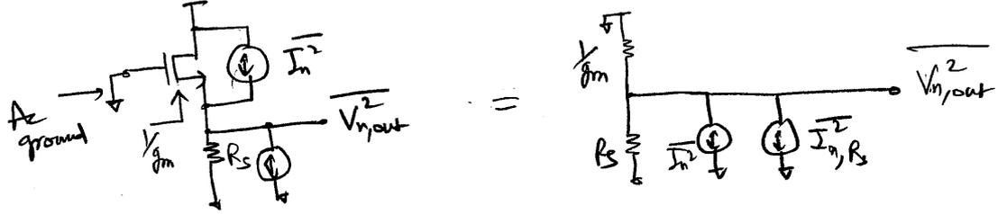
$$\overline{V_{n,out}^2} = (\overline{I_n^2} + \frac{4kT}{R_s}) (\frac{1}{g_m} \parallel R_s)^2$$
