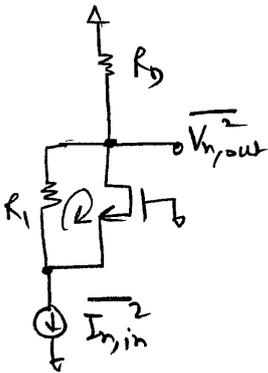
$$\overline{V_{n,out}^2} = \overline{I_{n,in}^2} R_D^2 \rightarrow \textcircled{2}$$
