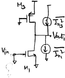
$$\Rightarrow \overline{V_{n,in}^2} = 2 \times \left( \frac{\overline{I_{n1}^2}}{g_{m1}^2} + \frac{\overline{I_{n3}^2} \cdot (r_{o1} \parallel r_{o3})^2}{g_{m1}^2 (r_{o1} \parallel r_{o3})^2} \right)$$
