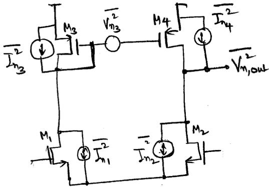
Most of the noise current  $\overline{I_{n1}}$  and  $\overline{I_{n3}}$  flows into  $M_3$  due to  $\frac{1}{g_{m3}}$  impedance
