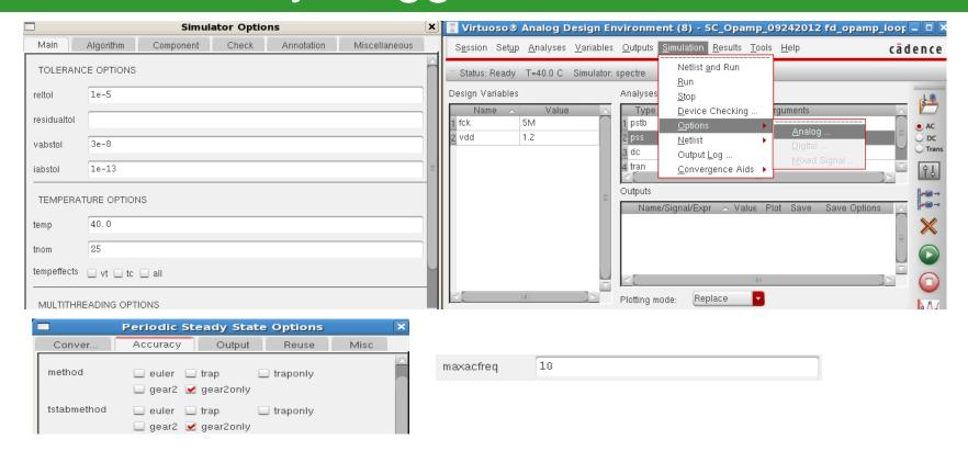
□ Go to Simulation →Options→ Analog →Main in the ADE window to setup tolerance options accordingly. If the frequency of periodic small signal analyses followed by PSS is high (e.g. 1G), the maxacfreq parameter (options→accuracy) of the PSS can be used to specify the highest frequency, otherwise, the frequency analysis in PAC maybe truncated.
