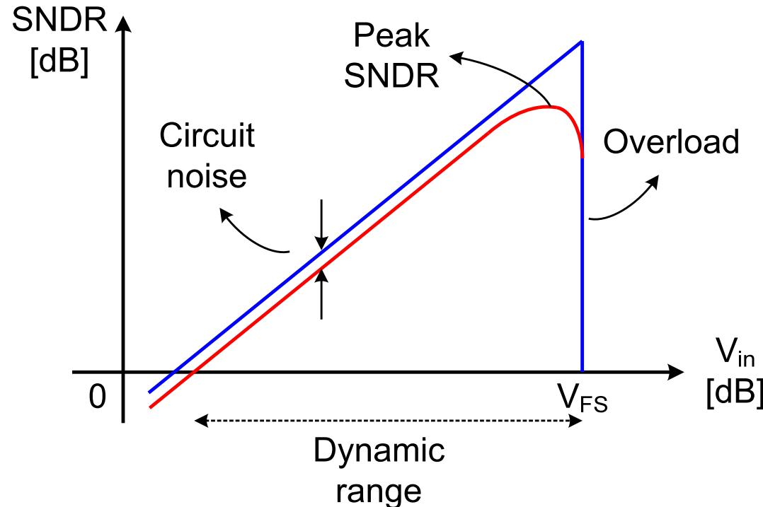
$$\begin{aligned} \text{SNR} &= 10 \log_{10} \left( \frac{V_{in}^2 / 2}{\Delta^2 / 12 + \sigma_N^2} \right) \\ &\propto V_{in} [\text{dB}] \end{aligned}$$
