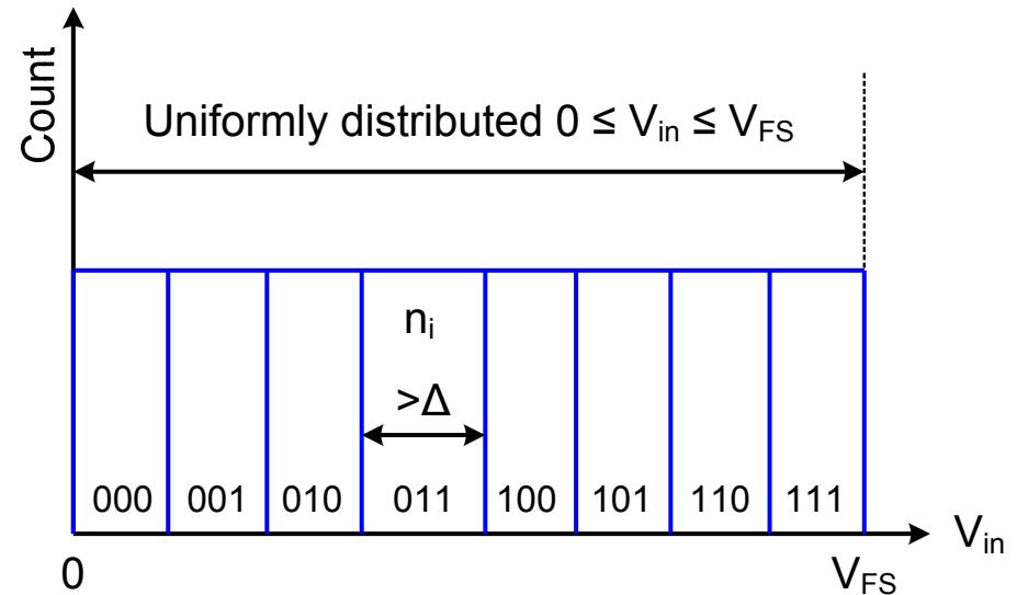
$$DNL_i = \frac{i^{\text{th}} \text{ Step Size} - \Delta}{\Delta} \approx \frac{n_i - \langle n_i \rangle}{\langle n_i \rangle}$$
