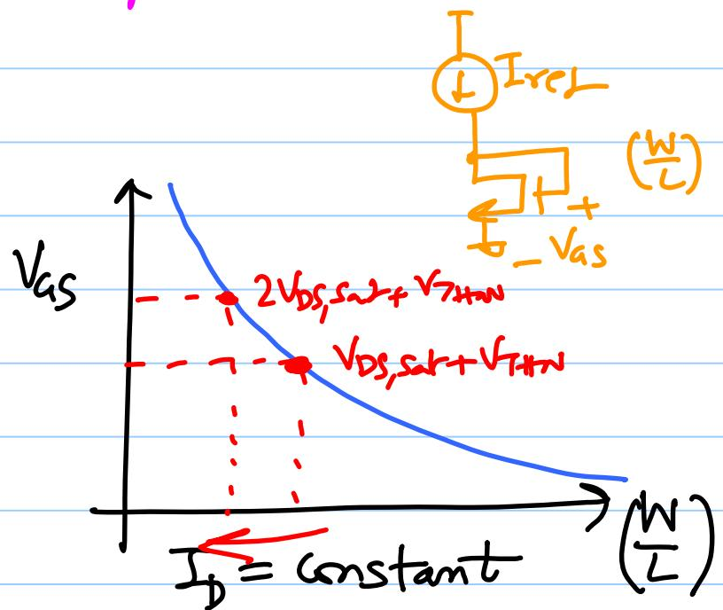
$$\begin{aligned} V_b &= V_{GS} + V_{DS,sat} \\ &= \underline{2V_{DS,sat} + V_{THN}} \end{aligned}$$
