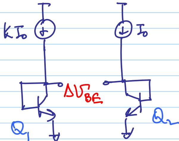
$$V_{BE1} \propto \ln(I_1/I_S)$$
