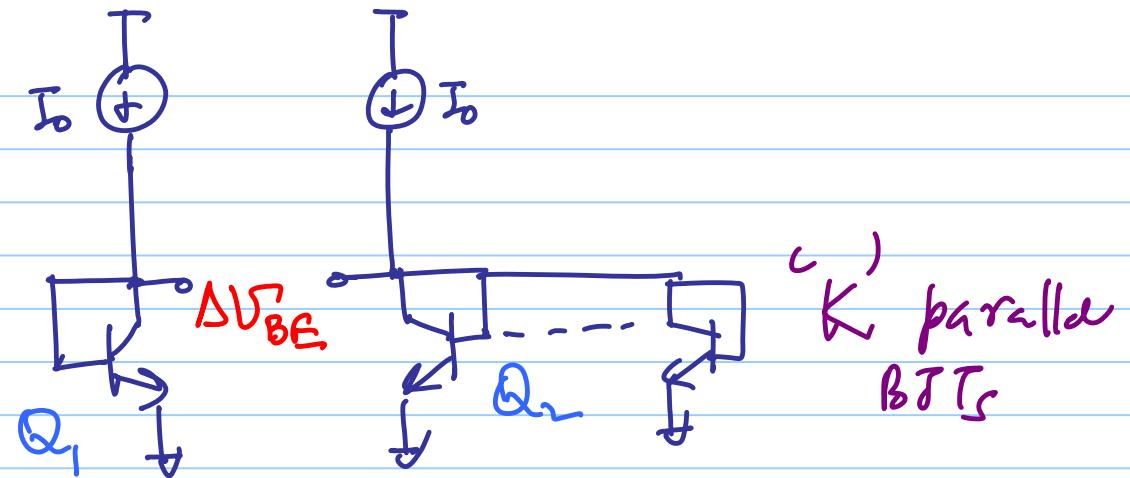
$$\Delta V_{BE} = V_T \ln \left( \frac{I_1}{I_2} \right) = V_T \ln \left( \frac{I_o}{I_o/k} \right) = V_T \ln(k)$$
