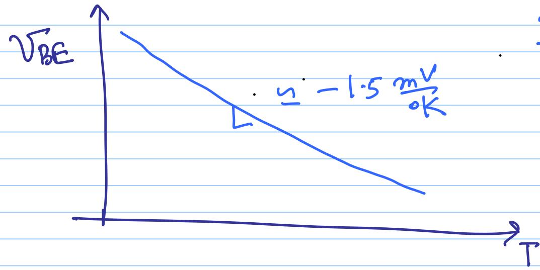
$$\frac{\partial V_{BE}}{\partial T} \approx -1.5 \frac{\text{mV}}{\text{K}}$$
