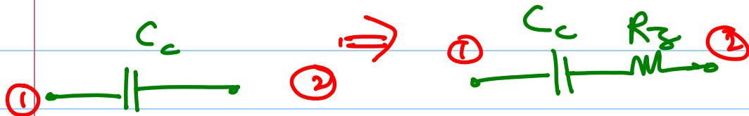
$$\omega_3 = \frac{1}{C_c \left( \frac{1}{g_{m1}} - R_2 \right)}$$
