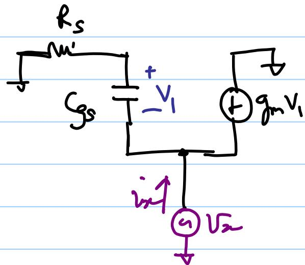
$$Z_{out} = \frac{V_2}{I_{out}} = \frac{R_s C_{gs} S + 1}{g_m + S C_{gs}}$$
