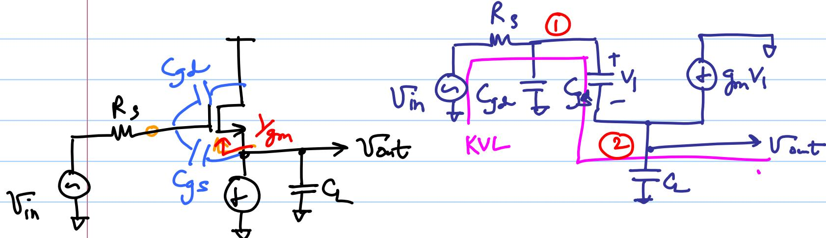
@ mode ②  $V_i C_{GS} + g_m V_i = V_{out} s C_L$
