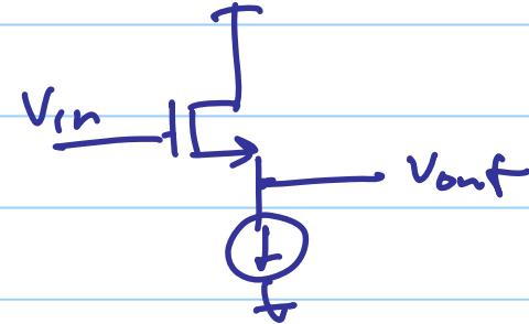
Voltage Buffer with DC level-shift
