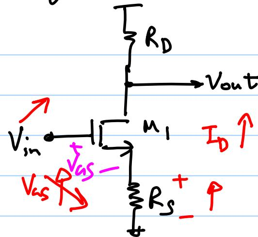
$$I_D = \frac{V_{in} - V_{gs}}{R_S}$$
