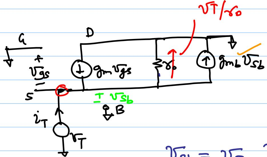
$$\left. \begin{aligned} V_{TSb} &= V_T \\ V_{gs} &= -V_T \end{aligned} \right\}$$
