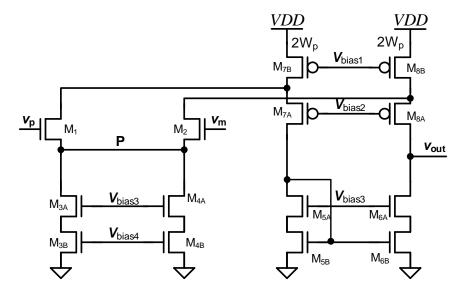
(a) (4 points) Assuming that **P** is an AC ground, draw the half circuits and find an expression for the small-signal differential gain  $(A_{v,DM} = \frac{v_{out}}{v_{in}})$ , where  $v_{in} = v_p - v_m$ . expression. Use variables  $g_{m1}$ ,  $r_{o1}$ ,  $g_{m5}$ ,  $r_{o5}$ , etc to show your work.
