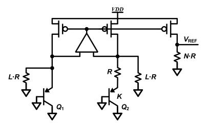
Given:  $\frac{\partial v_{BE}}{\partial T}=-1.5\frac{mV}{K},\;\frac{\partial v_{T}}{\partial T}=0.085\frac{mV}{K}$
