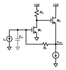
Ignoring channel length modulation and body effect ( $\lambda = 0$ ,  $\gamma = 0$ ), find the low-frequency, small-signal transimpedance ( $R_T$ ) defined as  $R_T = \frac{v_{out}}{i_{in}}$ .
