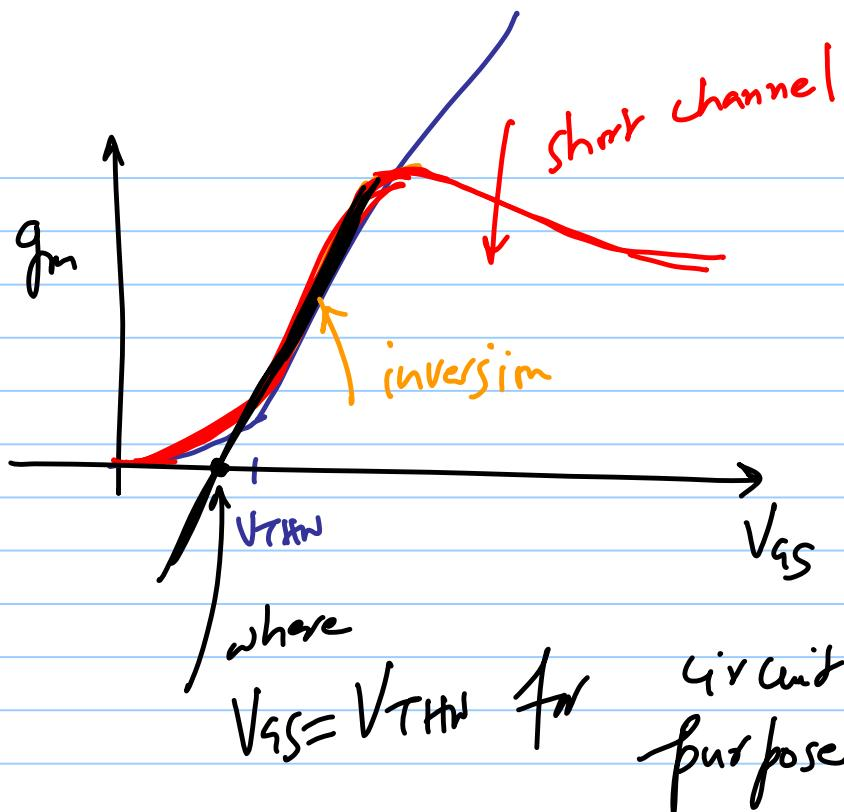
$$g_m = \beta(V_{GS} - V_{THN})$$
