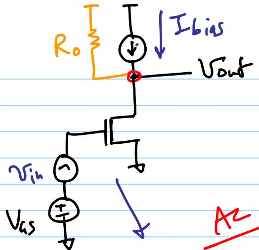
maximum gain of the transistor
