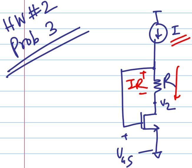
$$\begin{aligned} V_2 &= V_{AS} - V_{THN} \\ &= V_{AS} - IR \end{aligned}$$
