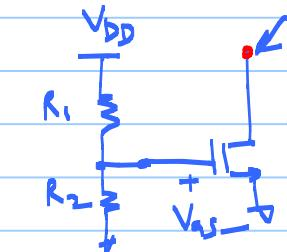
$$I_{out} = \frac{k_m}{2} \cdot \frac{w}{L} \left( V_{AS} - V_{THN} \right)^2 \quad (\text{initially } \gamma=0)$$
