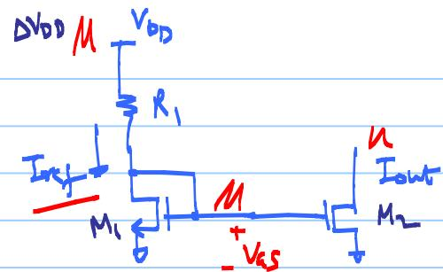
$V_{DD}$  ← Supply independent biasing
