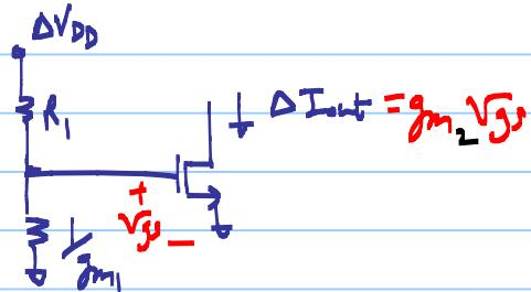
$$\checkmark \Delta I_{out} = \frac{\Delta V_{DD}}{R_1 + \frac{1}{g_{m1}}} \cdot \frac{(v/L)_2}{(v/L)_1}$$
