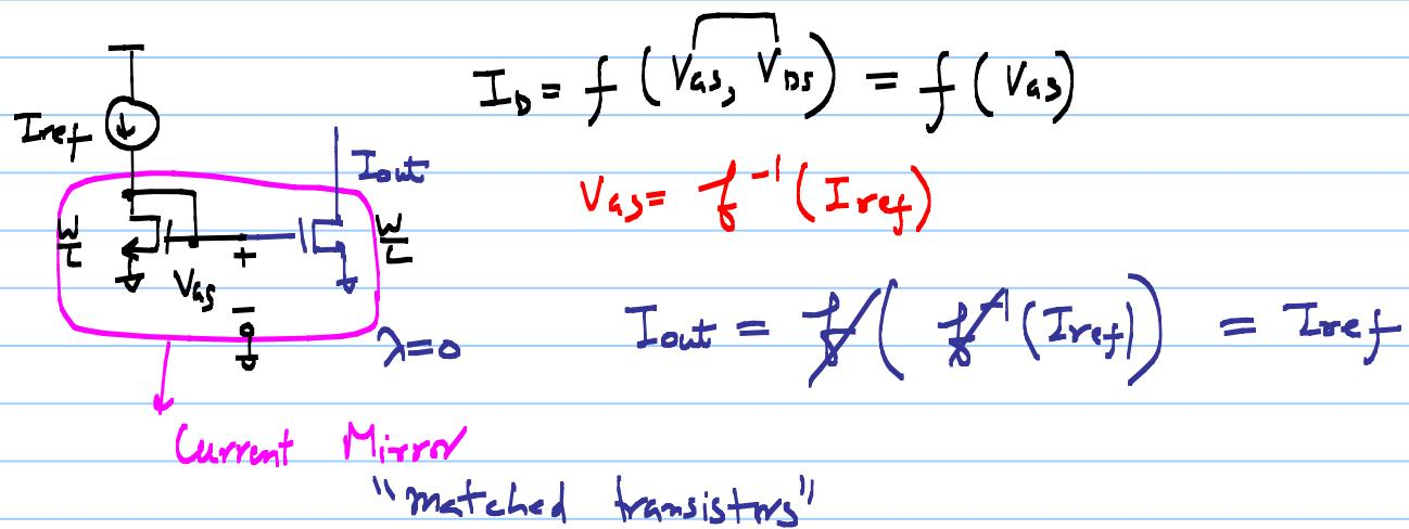
$$I_{ref} = \frac{1}{2} k P_m \left(\frac{W}{L}\right)_1 (V_{GS} - V_{THN})^2$$
