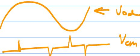
$\Rightarrow$  Differential signalling rejects "common-mode noise".
