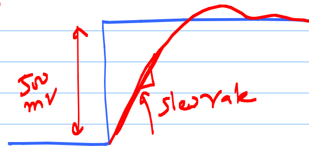
Figure 24.14 Good step response of the op-amp with the zero absent.
