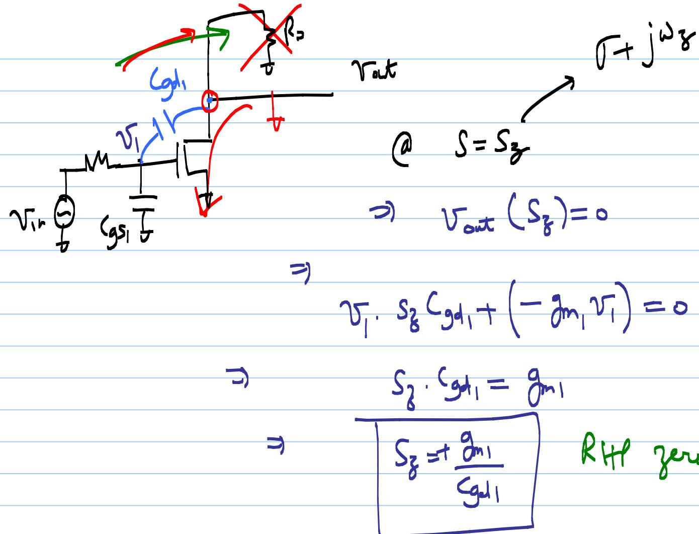
$$A(s) = A_V \cdot \frac{\left(1 - \frac{s}{\omega_3}\right)}{\left(1 + \frac{s}{\omega_{p1}}\right) \left(1 + \frac{s}{\omega_{p2}}\right)}$$
