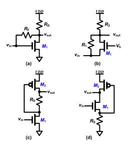
**Problem B2:** Assuming all transistors are in saturation, find small-signal voltage gain for each of the circuits shown below. Use variables  $g_{m1}$ ,  $r_{o1}$ ,  $g_{m2}$ ,  $r_{o2}$ , etc.
