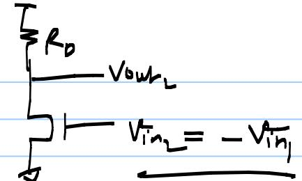
$$\frac{V_{out_1}}{V_{in_1}} = -g_{m1}(R_D || r_o)$$
