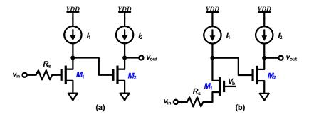
**Problem 2:** Calculate the input impedance and the small-signal transfer function for each of the circuits shown below (symbolic answers). For both the parts assume  $\lambda = \gamma = 0$ .
