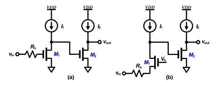
**Problem B4:** Calculate the input impedance and the small-signal transfer function for each of the circuits shown below (symbolic answers). For both the parts assume  $\lambda = \gamma = 0$ .
