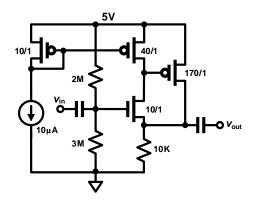
$V_{THN} = 0.7V$ , and  $KP_n = 200 \frac{\mu A}{V^2}$  $V_{THP} = 0.8V$ , and  $KP_p = 50 \frac{\mu A}{V^2}$  $\gamma = 0$
