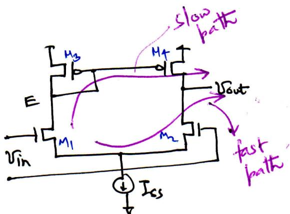
\* The topology contains two signal paths to the output with different transfer functions.
