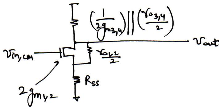
$$\Rightarrow A_{v,cm} = \frac{-\frac{1}{2g_{m3,4}} \parallel \frac{Y_{o3,4}}{2}}{\frac{1}{g_{m1,2}} + R_{ss}}$$
