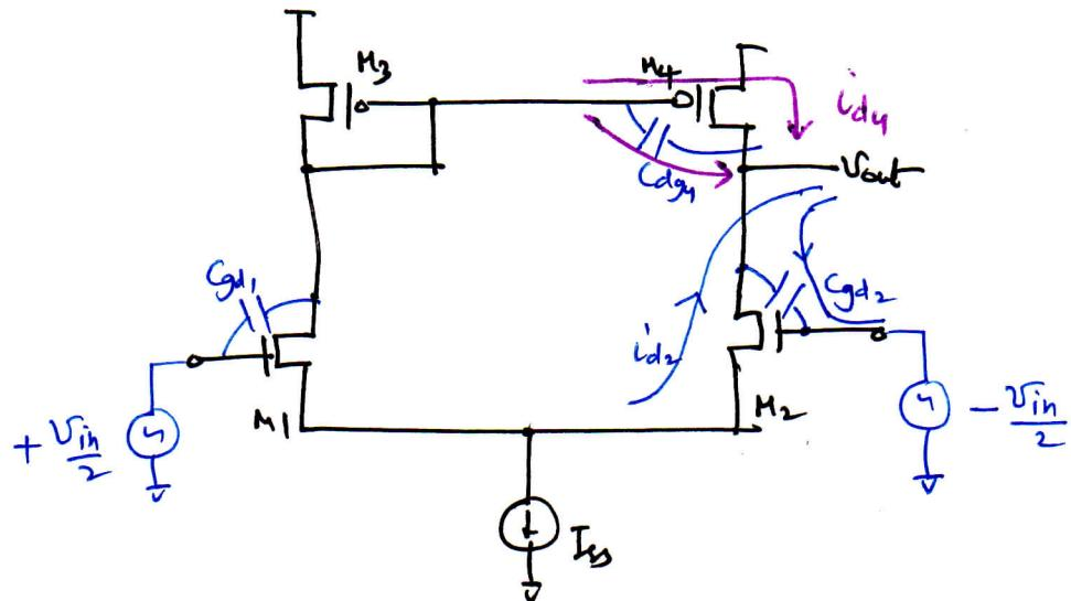
fast path : Currents adding in opposite polarity at the output
