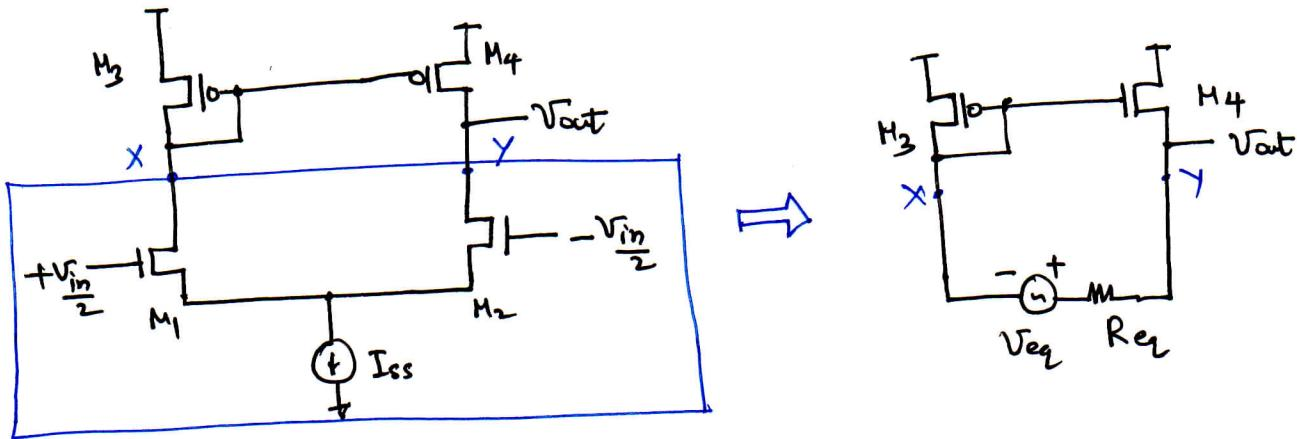
↳ Calculation of the Thvenin equivalent circuit.
