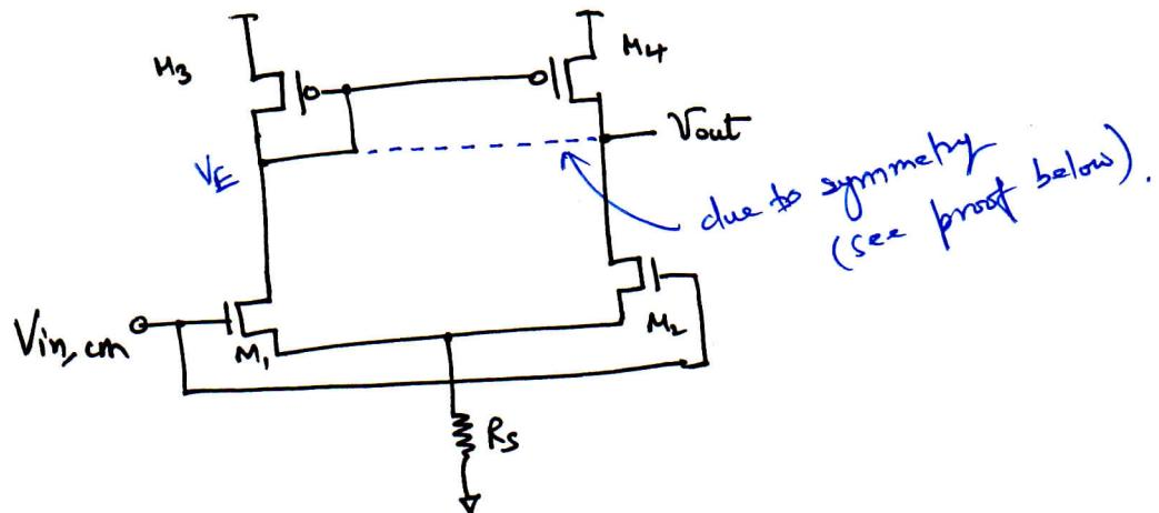
We first require to prove that the circuit is symmetric for CM analysis, i.e.  $V_{out}$  tracks  $V_E$ .
