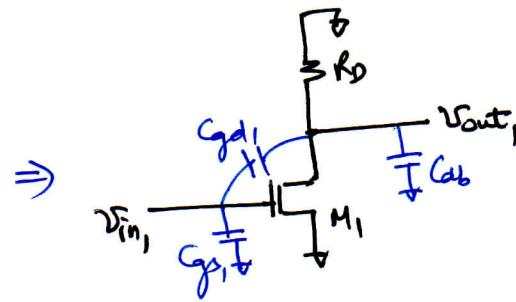
⇒ frequency response is same as the CS amplifier (with  $R_s = 0$ ).
