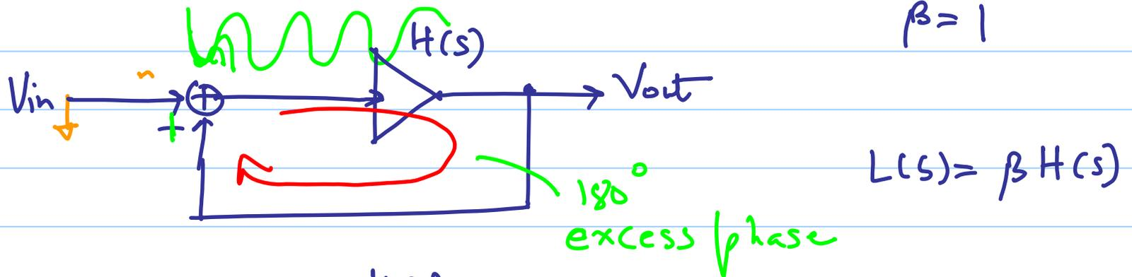
$$H_{cl}(s) = \frac{V_{out}(s)}{V_{in}} = \frac{H(s)}{1 + L(s)}$$
