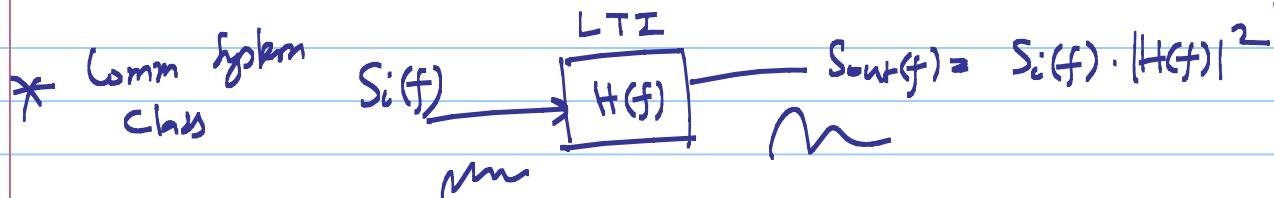
④ Determine the contribution of each noise source to the output  $\Rightarrow (H_i(f))^2 \cdot S_i(f)$
