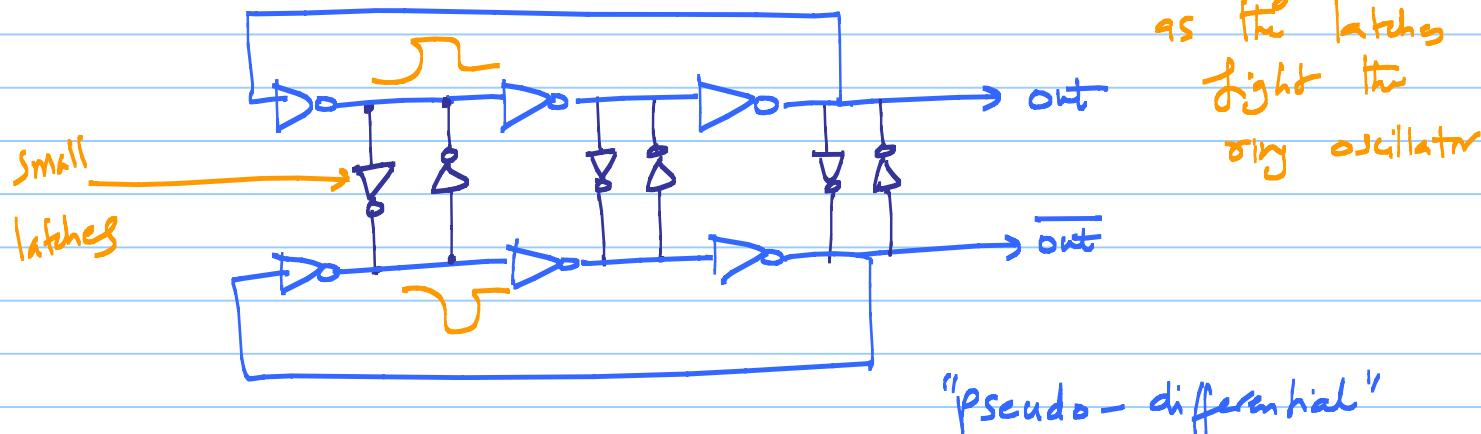
$V_{CO}$  with even delay steps
