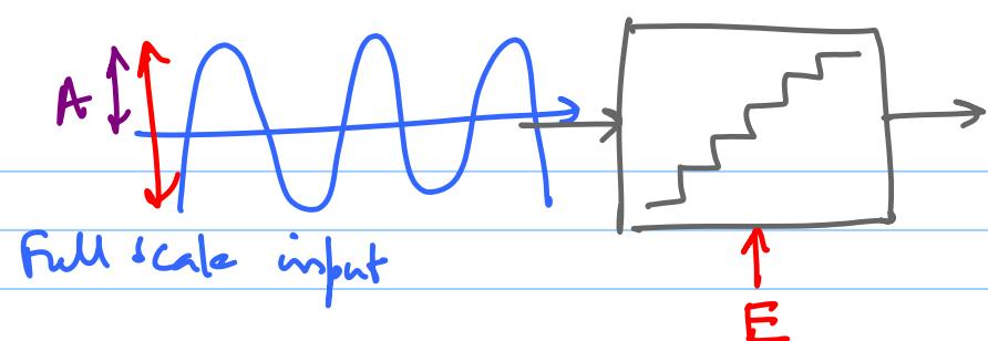
Signal to quantization noise ratio
