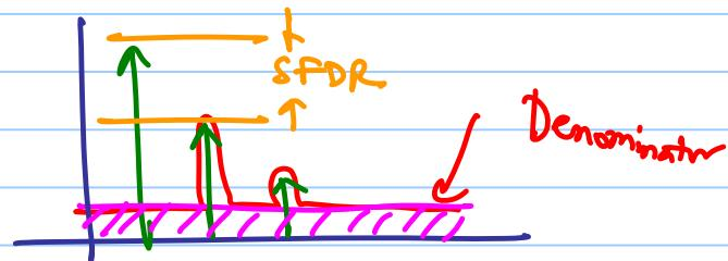
$$SFDR_{dB} = 10 \log_{10} \left( \frac{\text{signal power}}{\text{largest spurious power}} \right)$$
