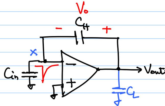
$$\tau_{amp} = \frac{C_L C_{in} + C_{in} C_f + C_f C_L}{g_m C_f}$$
