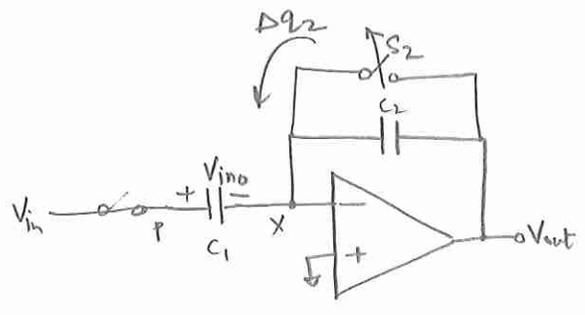
$\Delta Q_2$  is a constant charge injected into  $C_1$
