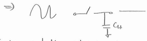
Track and hold capability of a sampling circuit.
