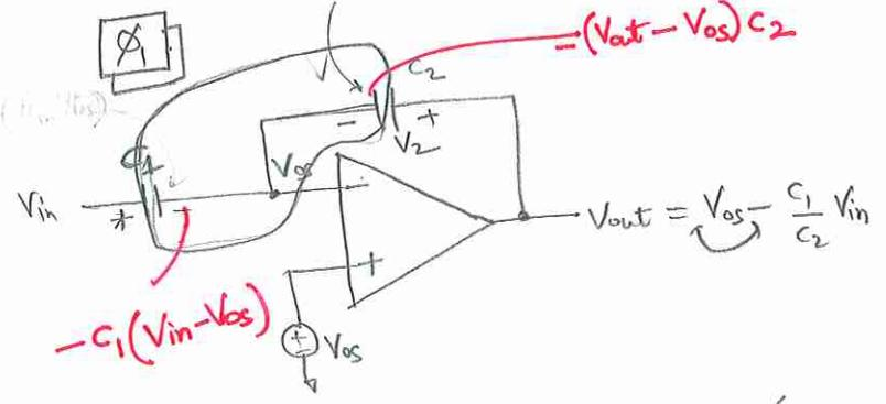
$$-C_1 V_{in} + C_1 V_{os} - C_2 V_{out} + C_2 V_{os} = C_1 V_{os}$$
