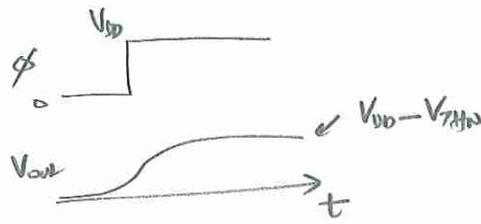
\* Eventually, subthreshold current will flow and  $V_{out}$  will reach  $V_{DD}$ .
