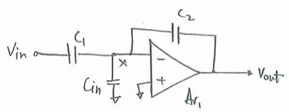
$$(V_{out} - V_x) s C_2 = V_x s C_{in} + (V_x - V_{in}) s C_1 \rightarrow \textcircled{1}$$
