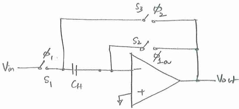
Circuit Trick for avoiding input dependent charge injection
