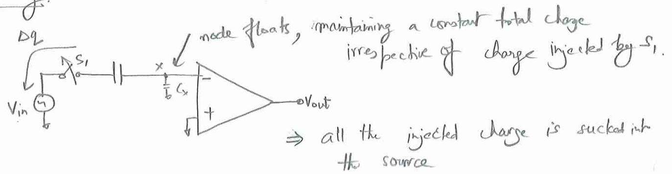
⇒ all the injected charge is sucked into the source
