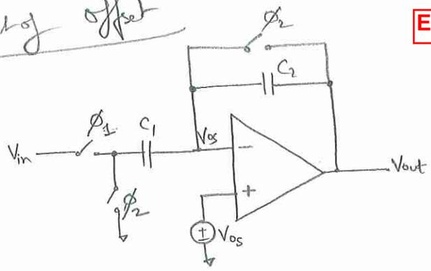
charge on  $C_1$  is  $+C_1(V_{in} - V_{os})$
