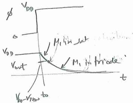
$V_{out} = V_{DD} \Rightarrow I_D(t_0) = \frac{\mu_n C_{ox} W}{2L} (V_{DD} - V_{TN})^2$
