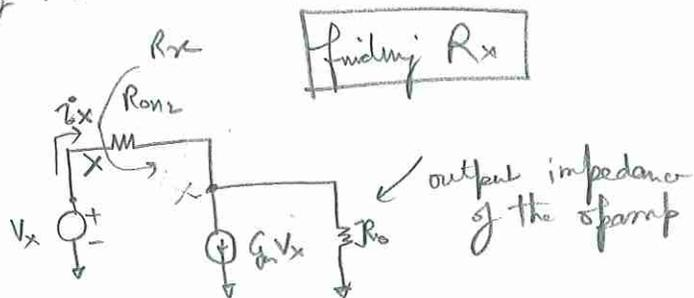
Total resistance in series with  $C_H \Rightarrow R_{on1} + R_x$  resistance between X and ground
