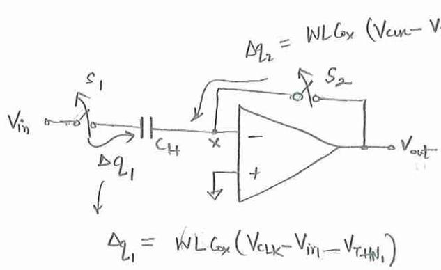
$$\Delta q_2 = WL C_{ox} (V_{clk} - V_x - V_{THN2}) \approx WL C_{ox} (V_{clk} - V_{THN1})$$
