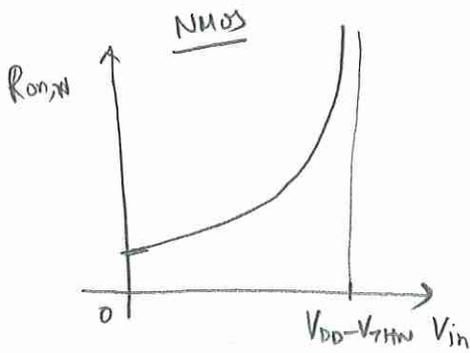
$$R_{on,n} = \frac{1}{\mu_n C_{ox} \frac{W}{L} (V_{DD} - V_{in} - V_{THN})}$$
