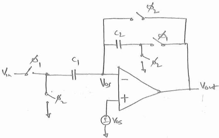
$\phi_2$ : charge  $C_2$  to the offset voltage instead of 0V
