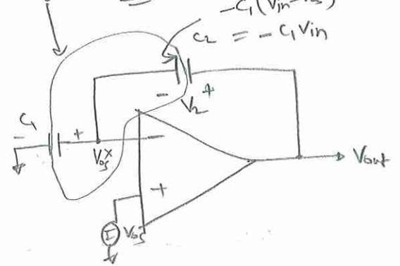
$$\Rightarrow -C_2 V_2 = -C_1 V_{in} (V_{in} - V_{os})$$
