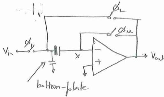
→ Bottom plate of the cap must be connected to the input to minimize  $C_{in}$
