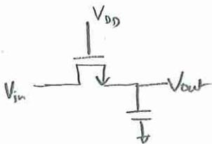
$$V_{DS} V_{GS} = V_{DD} - V_{out} = V_{DD} - V_{in}$$
