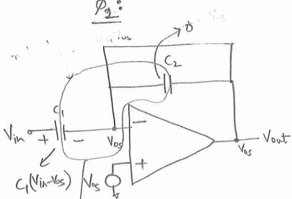
net charge on this surface =  $-C_1(V_{in} - V_{os})$
