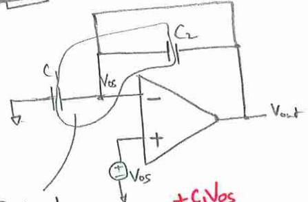
Total charge on the surface =  $+C_1 V_{os}$
