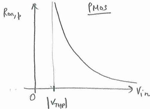
$$R_{on,p} = \frac{1}{\mu_p C_{ox} \frac{W}{L} (V_{in} - |V_{THP}|)}$$
