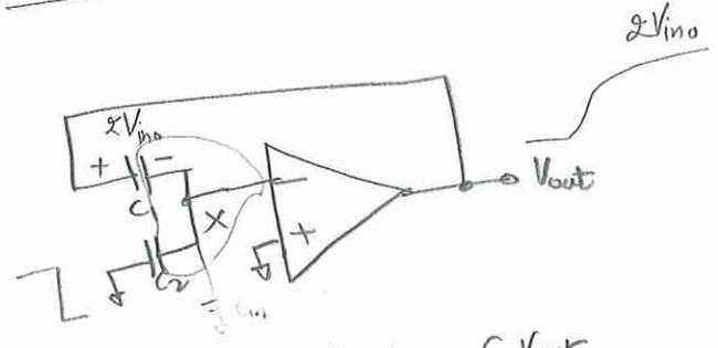
$-2V_{ino} \cdot C_1 = -C_1 V_{out}$
