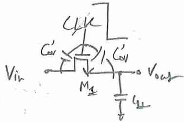
$\Delta V = V_{clk} \cdot \frac{W C'_{ov}}{N C'_{ov} + C_H}$  (overlap  $C_{ov}$ )
