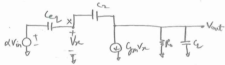
$$\Rightarrow V_x = (\alpha V_{in} - V_{out}) \frac{C_{eq}}{C_{eq} + C_2} + V_{out}$$
