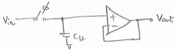
Here, Input dependent charge injection limits the accuracy. Will not work.
