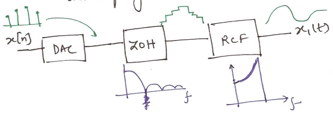
$\text{sinc}^{-1}$  response shape is used in the RCF to compensate for the Sinc distortion in the ZOH
